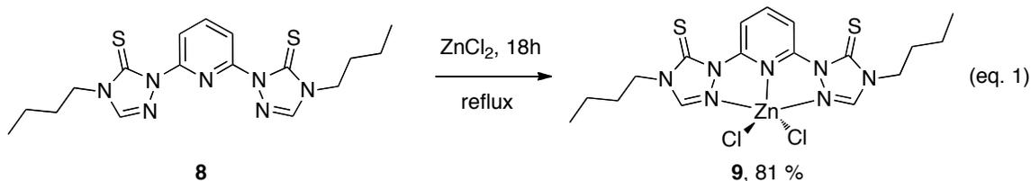
The driving force for the metallation is the formation of neutral zinc complex **9**, which is sparingly soluble in  $CH_2Cl_2$ . Off-white single crystals suitable for X-ray diffraction were grown by allowing diethyl ether vapor to slowly diffuse into an acetonitrile solution containing the zinc complex. All of the reactions (scheme 1 and eq. 1) were performed in air and proceeded with yields at or above 41 %. Zinc complex **9** is soluble in dimethyl
