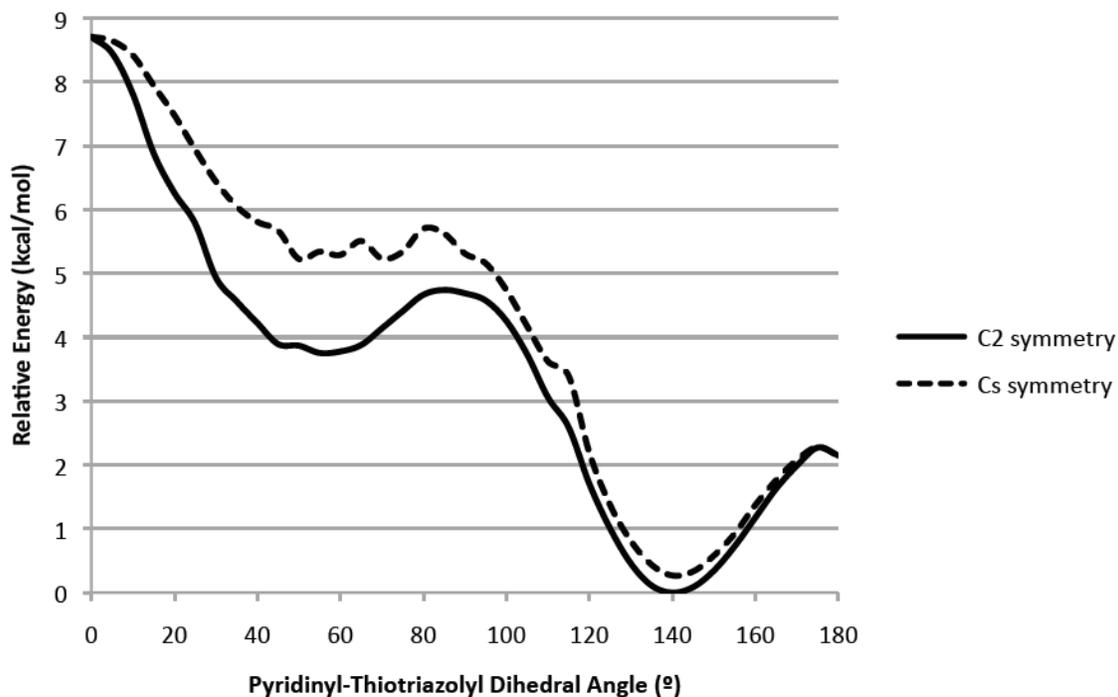
**Fig. 5.** Relative total energy vs. pyridinyl-thiotriazolyl dihedral angle for 2,6-bis{[N-methyl]triazole-1-ylidene-2-thione}pyridine modeled under C<sub>2</sub> and C<sub>s</sub> symmetries.
