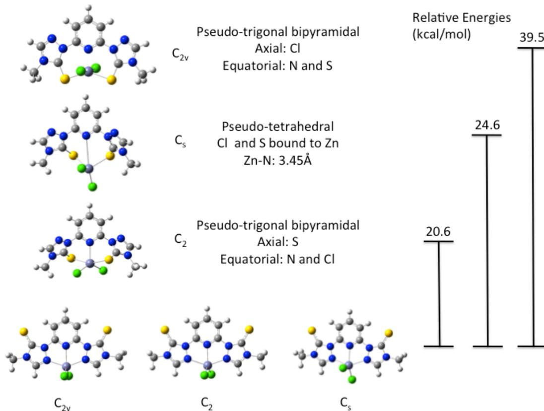
**Fig. 7.** Various geometry-optimized conformations of dichloro(η<sup>3</sup>-N,N,N)-[2,6-bis(3-[N-methyl]triazol-5-thione-1-yl)]pyridinezinc(II) and their relative energies.
