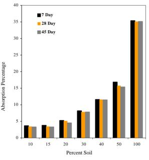
Figure 1. Absorption percentage as affected by soil content.
