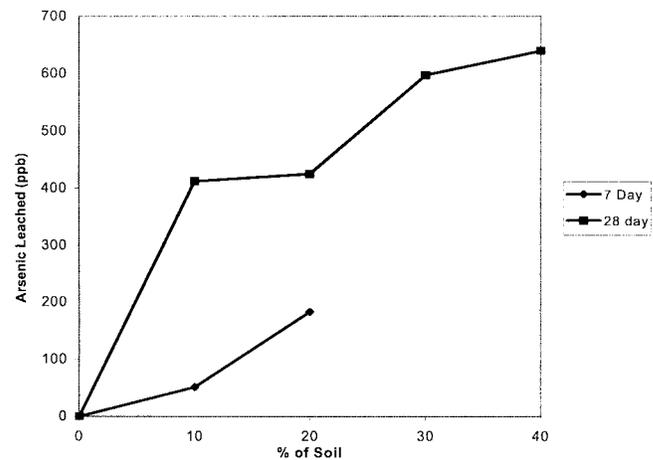
Fig. 14—TCLP results as affected by soil content.
