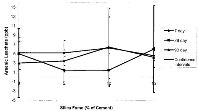
Fig. 12—TCLP as affected by silica fume content.
