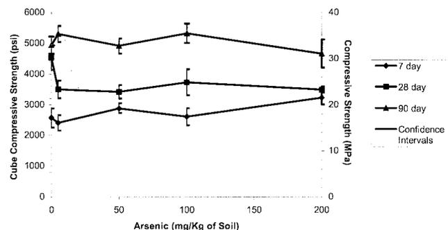
Fig. 3—Compressive strength as affected by arsenic content.
