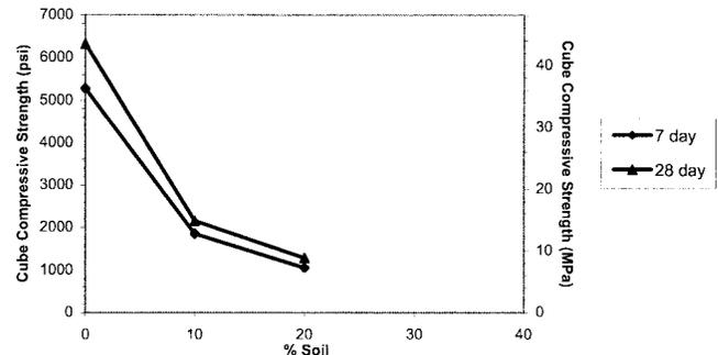
Fig. 13—Compressive strength as affected by soil cement.
