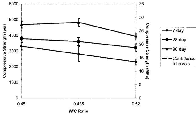
Fig. 5—Compressive strength as affected by w/c.
