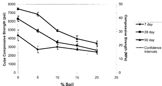
Fig. 2—Compressive strength as affected by soil cement.
