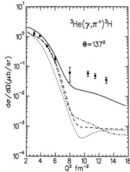
FIG. 2. Differential cross section at  $\theta_{\pi}^{\text{c.m.}} = 137^\circ$  as a function of nuclear momentum transfer  $Q^2$  from Ref. [3]. The dotted (dashed) curves show the PWIA (DWIA) results. The dash-dotted curve includes the corrections due to coupling with the breakup channels, and the solid line shows the complete calculation with the additional two-body mechanisms. Figure is from Ref. [10].
