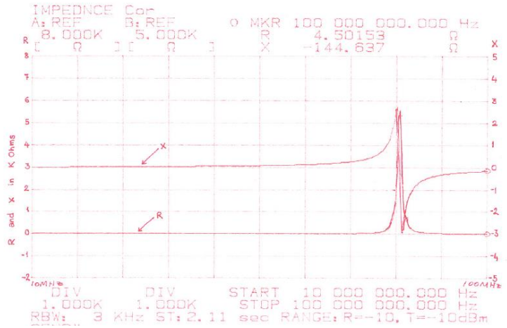
Fig. 3 Input impedance of a cable terminated in short circuit
