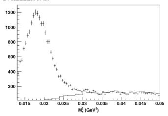
FIG. 11. Missing mass of  $\gamma p \to K^+ \Lambda(X)$  for data (points with error bars) and Monte Carlo simulations for the  $\gamma p \to K^+ \Lambda(1405)$  reaction (histogram) normalized to the data.
