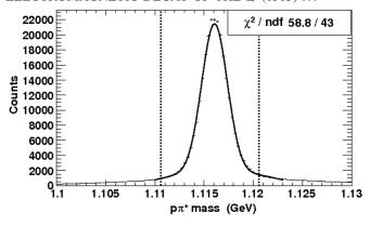
FIG. 3. The invariant mass of the p- $\pi$ <sup>-</sup> showing the  $\Lambda$  peak with a Gaussian fit giving a  $\sigma=1.3$  MeV. A cut of  $\pm 0.005$  GeV around the Particle Data Group mass of the  $\Lambda$  is used indicated by the dotted lines.
