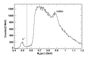
FIG. 5. Missing mass for the reaction  $\gamma p \to \Lambda(X)$  for events passing cuts on the  $\Lambda$  and  $\Sigma^*$  masses. The dotted line at 0.55 GeV shows the cut used to remove the  $\gamma p \to K^+ \Lambda$  channel. (A looser timing cut was used to illustrate that these accidentals are at the  $K^+$  mass.)
