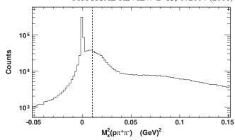
FIG. 1. Missing mass squared  $(M_x^2)$  for the reaction  $\gamma p \to p \pi^+ \pi^-(X)$ , where the  $\pi^+$  was a potentially misidentified kaon. Events above the dotted line at 0.01 GeV<sup>2</sup> were kept.
