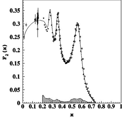
FIG. 6. Structure function  $F_2(x, Q^2)$  at  $Q^2 = 0.775 \text{ GeV}^2$ ; stars represent experimental data obtained in the present analysis with systematic errors indicated by the hatched area, open circles show data from previous experiments [7,30–44] and the solid line represents the parametrization from Ref. [14].
