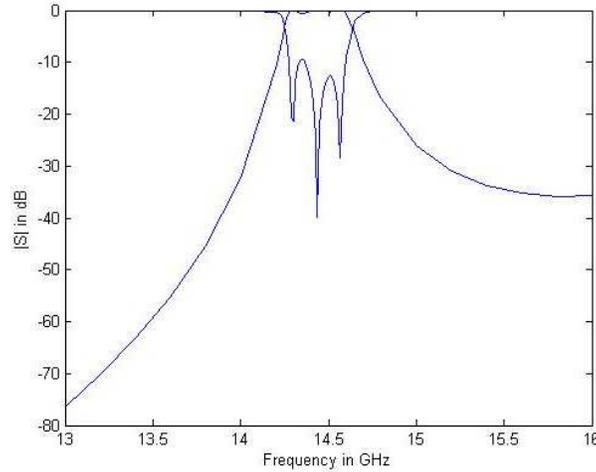
Figure 5: Response of the filter. Input and output rectangular waveguide of dimension  $1.58 \times 0.79$  cm, Cavity radius = 0.6985 cm, Iris thickness = 0.127 mm, cavity lengths = 1.91, 1.97, 1.91 cm.
