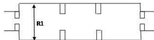
Figure 2: Filter structure showing irises of finite thicknesses.
