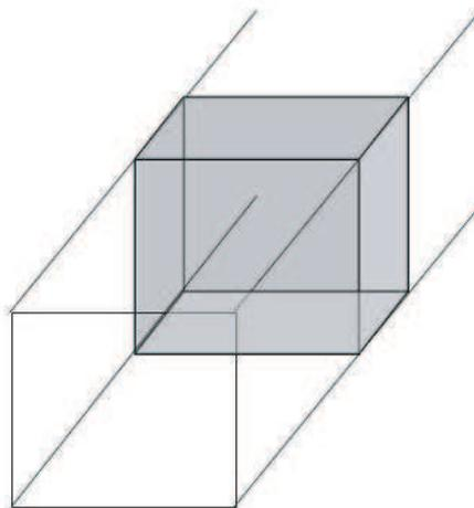
Figure 1: Dielectric sample in cross-section of waveguide.
